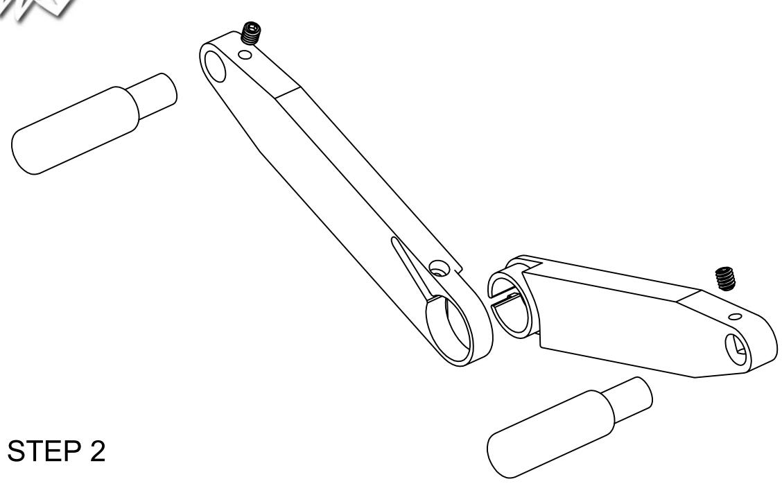
Place the Rubber Coated Rods into each Arm and make sure they are flush on the back side.
